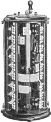
TYPE RF— DRUM CONTROLLER SECONDARY ONLY
